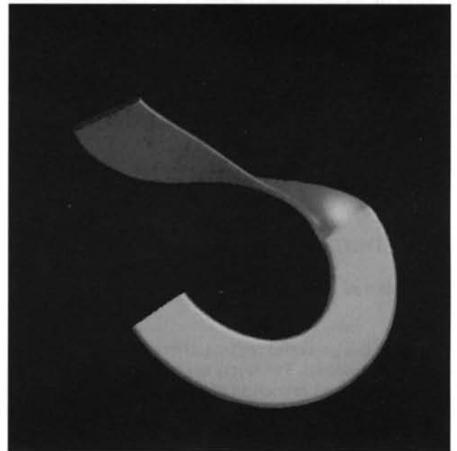
Figure 2 A G^0 surface generated by the Frenet frame along a C^2 cubic spline curve
